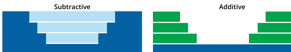
Fig. 6: left: subtractive process (dark blue: desired Part, light blue: removed material) | right: additive process (dark blue: base layer, green: added up layers) © PFI
