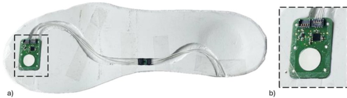
Fig. 19: a) Insole with humidity sensor and temperature sensor b) Zoom view of the humidity sensor. PFI (2022–2024). Safety of footwear containing electronic components under the Electronic Equipment Act (IGF project 22292 N).
