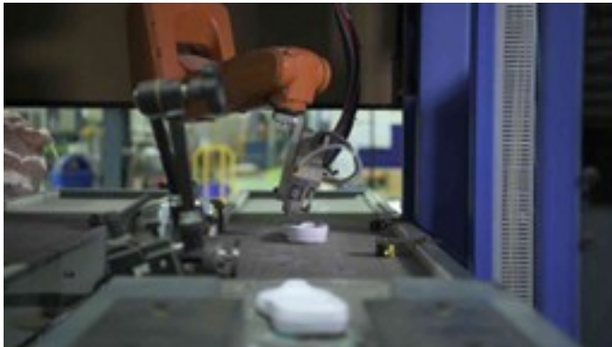
Fig. 48: Robot in lasting sector, applying glue in soles. Credit: Autecautomation
