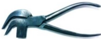
Fig. 42: Lasting pliers: tool to adjust the height of the shoe
