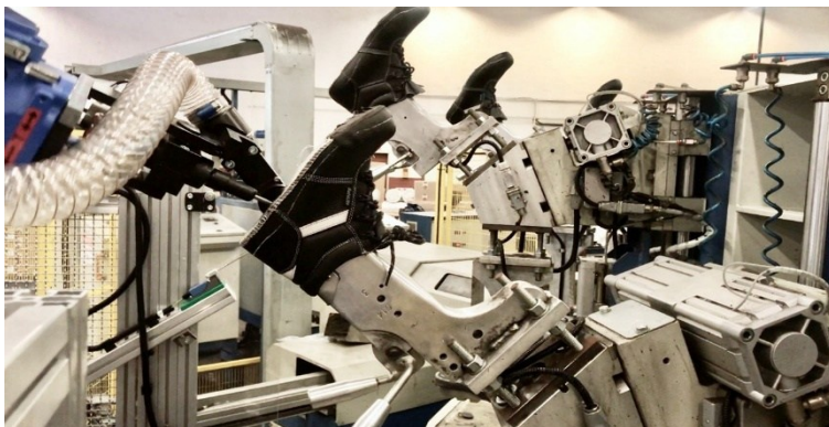
Fig. 47: Robot in lasting sector. Credit: Autecautomation
