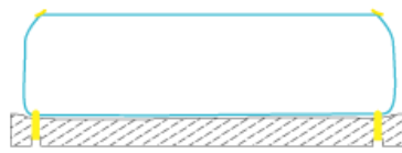
Fig. 15: Scheme of the moccasin lasting
