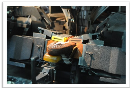
Work-based learning / Heat setting machine; Source: Carité
