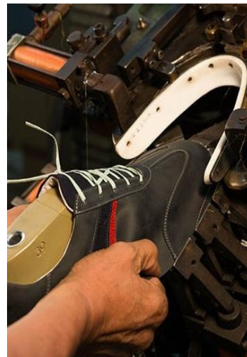
Fig. 39: Centre the shoe in relation to the pincers and teflon
