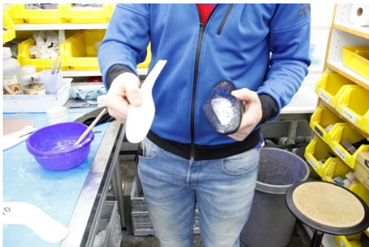
Fig. 9: The bottom filler's function is to level out the difference in height between the lasting edge and the insole. Credit: Gabor
