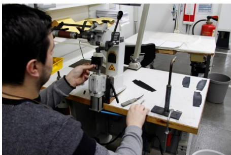
Fig. 12: Clamping device used for covering heels with leather. Credit: Gabor
