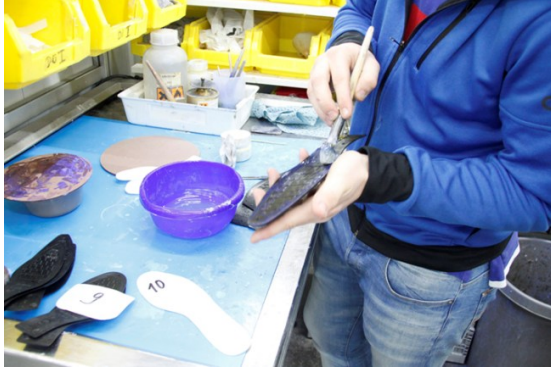
Fig. 10: Cement is applied to the sole. Credit: Gabor
