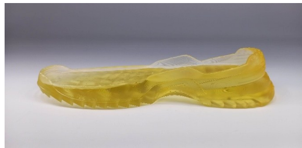
Fig. 22: Sole 3D printed – Credit: Solidator
