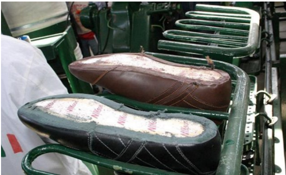
Fig. 6: If roughing dust remains on the roughed surface, it will be covered with glue in the next step, which will ultimately weaken the bonding strength. Credit: ISC
