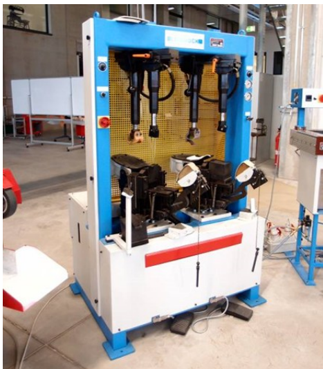
Fig. 17: Hydraulic sole press. Credit: ISC
