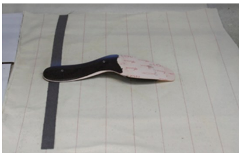
Fig. 14: Insole and piping strip to be glued around the edge. Credit: Gabor
