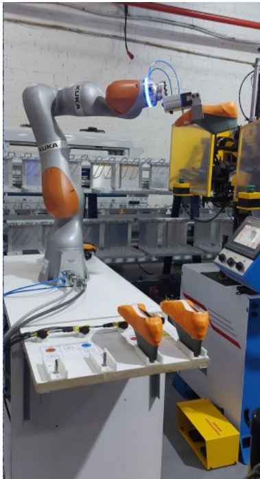
Fig. 20: Shoe assembly robot – Credit: https://serma.net/noticias/ferias/fimec/fimec-ratifico-el-buen-momento-de-brasil
