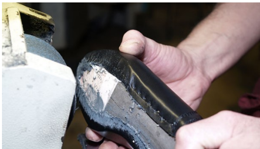
Fig. 2: Manual roughing (coarse sand paper). Credit: ISC
