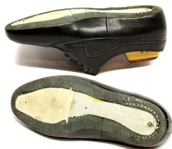
Fig. 4: Perfect roughing result: Only the grain layer has been removed. The structural strength of the upper leather is maintained and the contact area for the adhesive bond has been enlarged. Credit: ISC
