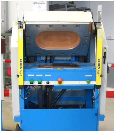
Fig. 18: Double membrane pneumatic sole press. Credit: ISC
