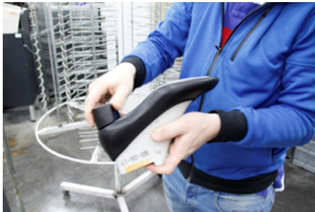
Fig. 13: This is what the covered heel will look like on the shoe. Credit: Gabor
