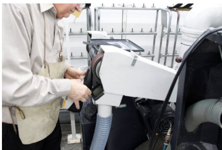
Fig. 3: Manual roughing (finer sand paper). Credit: Gabor
