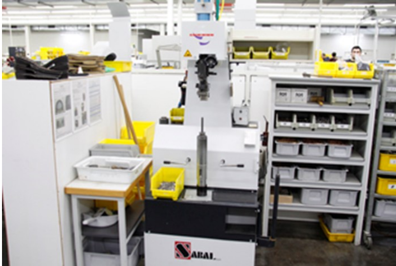
Fig. 19: Machine for screwing on heels. Credit: Gabor
