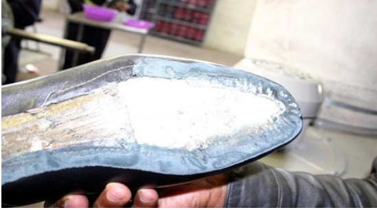
Fig. 5: Example of an over-roughed upper: the white interlining is showing through. The strength of the sole bond will now completely depend on the structural strength of lining and interlining. Credit: ISC
