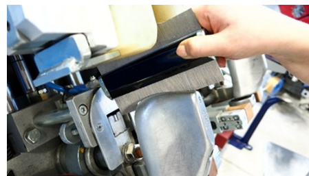
Fig. 7: Shape of mould must be identical with last shape © PFI
