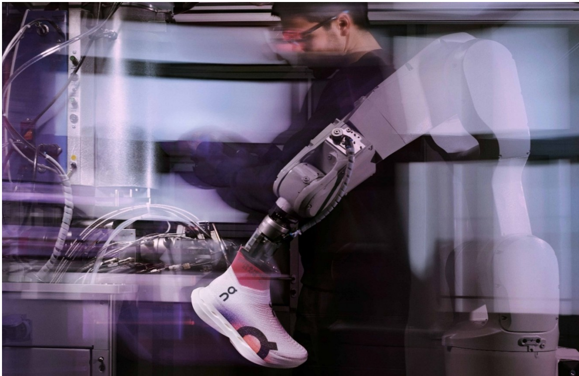
Fig. 14: On - Light Spray model of footwear with the upper done in 3 minutes. Source: https://www.gearpatrol.com/fitness/on-lightspray-running-shoes/
