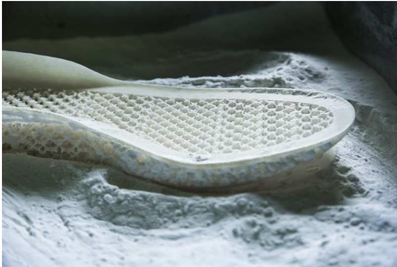
Fig. 26: Adidas 3D-printed running shoe midsole. Source: https://news.adidas.com/futurecraft/adidas-breaks-the-mold-with-3d-printed-performance-footwear/s/8099a318-f9e7-45d8-9887-42c3dde5e6fd
